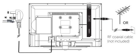
1. Connect one end of the RF coaxial cable to the aerial socket on the wall and the other end of the cable to the aerial socket at the rear bottom of the TV.
