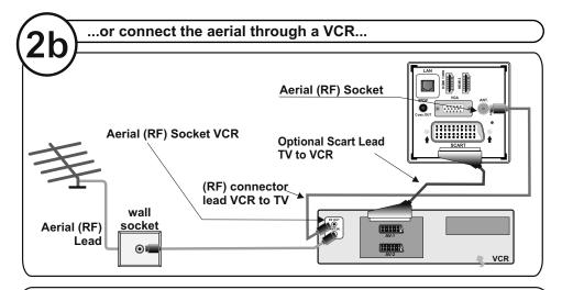
• It is recommended that a scart lead should be fitted between your TV and VCR to enhance your picture and sound quality. Scart leads are essential if you have a stereo TV and VCR and wish to obtain stereo sound from your equipment. These leads can be purchased from your Hitachi dealer or any good High Street electrical retailer.
