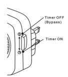
You can bypass the timer at any time by sliding the side switch to "Timer OFF" position for continual ON operation.
