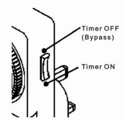
You can bypass the timer at any time by sliding the side switch to "Timer OFF" position for continual ON operation.
