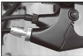
APPLY THE BRAKES TO CUT THE POWER AND STOP. FRONT BRAKE IS OPERATED BY RIGHT HAND BRAKE LEVER, REAR BRAKE IS OPERATED BY LEFT HAND BRAKE LEVER.
