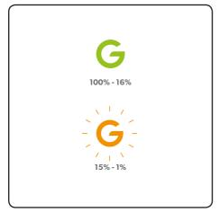
The battery indicator shows how much charge remains in the HyLite battery.
