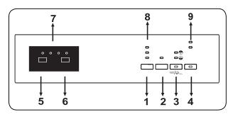
Press the On/Off button (4), to switch on the machine. The On/Off lamp remains lit when the machine is on.
