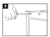
2. With the door closed remove the screws on the outside of the hinges. Start with the top hinge.
