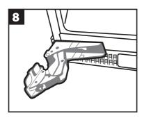
9. Check that the larder fridge door is aligned horizontally and vertically and that the door seals are secure on all sides before finally tightening the hinge bracket screws.
