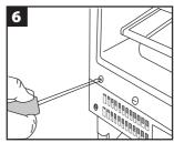
7.Turn the hinge over and place it on the diagonally opposite comer of the cabinet. Screw back in place.
