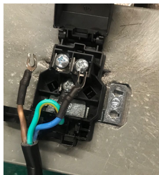
Fasten the wires beneath the screw heads
