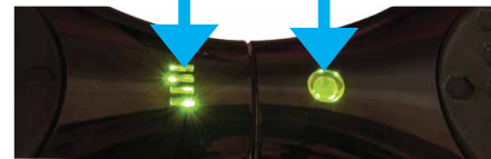
(A) Battery power level indicator (B) Balance level indicator
