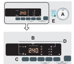
**A-Programme Selector -** Rotating the knob in both directions it's possible to select the desired drying program. To switch or cancel off the dryer rotate the knob on OFF.
