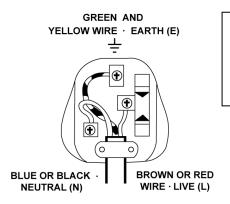
The wires in this mains lead are coloured in accordance with the following code:
