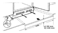
o Use a spanner to adjust the height of the adjustable feet.
