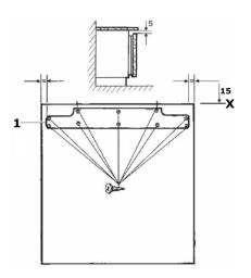
Measure the width of the furniture door, at the halfway point mark a line vertically down the inner surface of the furniture door. You should draw the line from the top of the furniture door to approximately halfway down.
