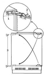
o Slacken the retaining screws (1) on the appliance and then carefully remove the appliance door.
