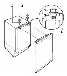
3. Hang the furniture door onto the appliance door, making sure that the brackets on the mounting bracket locate over the adjusting bolts.
