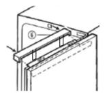
6. Insert the cover plate to the top of the appliance, this will just clip into place.
