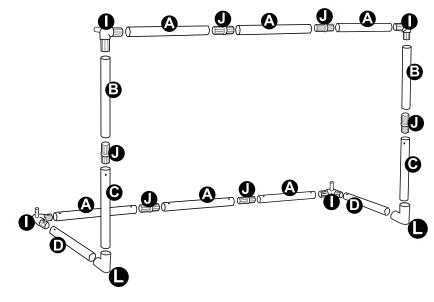
Join the tubes together with connectors as illustrated.
