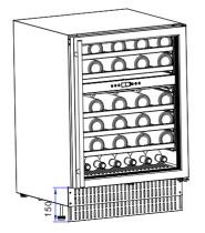
The plinth could be adjusted from 90mm to 150mm.
