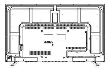
This equipment is a Class II or double insulated electrical appliance. It has been designed in such a way that it does not require a safety connection to electrical earth.
