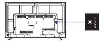
**Tip**: If you are using an antenna with a 300 ohm twin-lead cable, you need to use a 300-75 ohm adapter (not provided) to adapt the cable to a connection that is compatible with the TV's antenna input.
