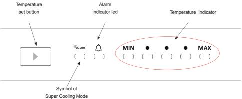
This button allows setting temperature of the fridge. In order to set values for fridge partition, press this button. Use this button also to activate Super Cooling mode.
