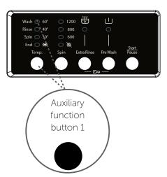
Use the washing water temperature adjustment button to alter the automatically programmed washing water temperature.
