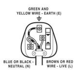
The BLUE wire must be connected to the terminal marked with the letter N
