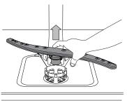
The lower spray arm may be removed by pulling it upwards.
