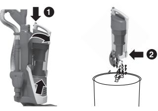
To remove the bin from the product, press the bin release button (1) and lift the bin unit away from the product. Hold the bin over the trash bin and press the bin empty button (2) the bin flap will open and the debris will empty into the trash with no dust contact. Once emptied, gently tap or shake the bin to release excess dust.
