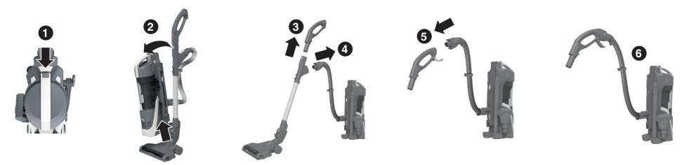
Release the main body unit by pressing the lift out button (1) and lifting the main body unit out and upward (2). Remove the handle form the tube (3), remove the power hose from the tube (4), fit the power hose to the handle (5).
