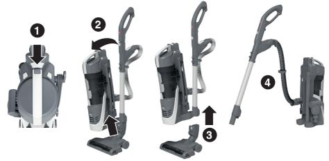
Release the main body unit by pressing the lift out button (1) and lifting the main body unit out and upward (2). Remove the power nozzle from the cleaner by pressing the nozzle release button (3).
