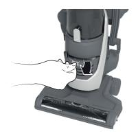
Remove the exhaust filter grille from the cleaner (1).
