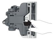
3 Remove brush assembly and check for wear on the belt.
