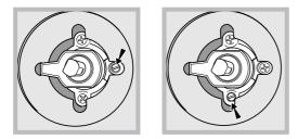
**!** After adjusting the appliance so it may be used with a different type of gas, replace the old rating label with a new one which corresponds to the new type of gas (these labels are available from Authorised Technical Assistance Centres).
