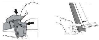
**2.** Lift and firmly hold the inner glass with both hands, remove it and place it on a soft surface before cleaning it.
