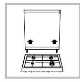
If the cooker is fitted with a glass cover, this cover should be cleaned using lukewarm water. Do not use abrasive products. It is possible to remove the cover in order to make cleaning the area behind
