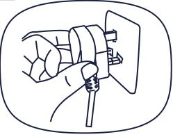
ii. Insert the battery pack along the support rails of the charger.
