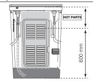
gas supply must be connected to the left of the appliance. Be sure that the hose does not pass through the rear of the cooker touching hot parts.
