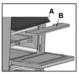
Slide the grill pan along the runner towards the rear of the grill compartment until it stops. An odour may be noticed when first using the grill - this schould cease after a short period of use.
