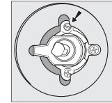
• check that the burner does not turn off when you turn the knob from Max to Min and and when you open and close the oven door quickly.
