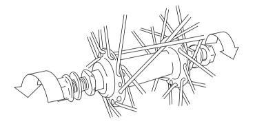
Make sure the wheel nuts are loosened by turning anticlockwise, exposing as much of the thread as possible.
