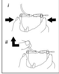
CABLE GUIDE PIPE (NOODLE) — Hooks into the left hand arm and connects the two brake arms so that they both move towards the wheel when the brake lever is pulled
