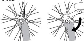
*iii* Place the pointed side of the locking washer into the hole in the fork as shown, then ensuring the gap between the wheel and the fork is equal on both sides, tighten the nut by turning clockwise using a spanner. Recommended torques can be found at the back of this catalogue
