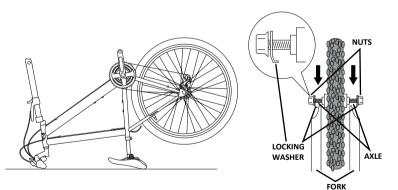
*ii* For this step, as long as your saddle and handlebar are installed, it helps to turn the bike upside down. You should then insert the wheel into the dropouts as shown, ensuring that the locking washers are on the outside of the fork as shown.
