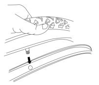
Always check that the rim tape is even around the rim and check the rim for any damage.
