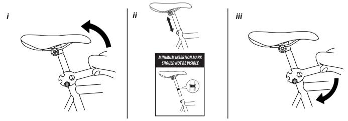
When adjusting the saddle, always be aware of the minumum insertion mark and always make sure this is not visible above the frame, or you risk damaging the bicycle or losing control causing serious injury or worse.
