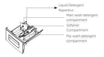
• Use detergents produced for automatic washing machine in your machine. The amount of detergent you will use for your laundry is printed on the detergent package.
