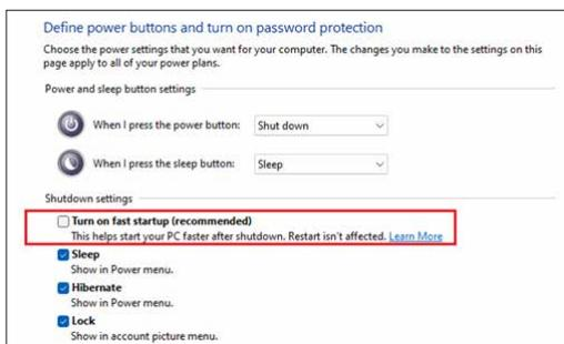
If fast startup is disabled, when you shut down the computer, it shuts down to the S5 power state.
