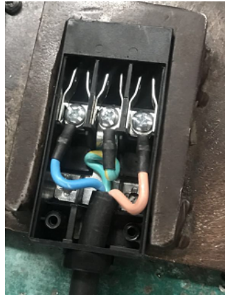
Fasten the wires beneath the screw heads
