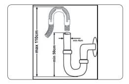
Connect water drain hose directly to water drain hole or to the sink outlet spigot. This connection should be minimum 50cm and maximum 110cm from floor plane.
