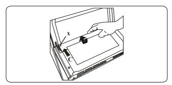
If the oven door is a triple glass oven door, the third glass layer can be removed the same way as the second glass layer.
