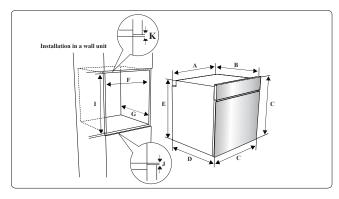
After making the electrical connections, insert the oven into the cabinet by pushing it forward. Open the oven door and insert 2 screws in the holes located on the oven frame. While the product frame touches the wooden surface of the cabinet, tighten the screws.
