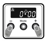
1. Press the "+" and "-" keys simultaneously. Symbol will appear, and the dot in the middle of the screen will start to flash.
