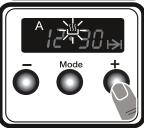
**6.** Select the desired finishing time using the "+" and "-" keys.
