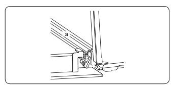
**3.** Close the door until it is almost in the fully closed position, and remove the door by pulling it towards you.
