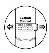
**3** The Suction Control slide. located at the base of the top handle, offers variable suction based on your needs. Slide toward MIN to minimise suction, and slide toward MAX to maximise suction.
