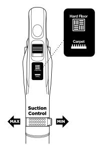
2 The soft roller spins in both settings to pick up extra dust and debris. Choose the appropriate setting:
