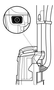
**3** Press power button to turn vacuum on to start cleaning. Please note the brushrolls will not spin unless the wand is reclined.
