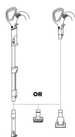
2 Insert desired tool directly onto wand or handle.
