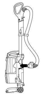
**3** Place pod onto wand and **4** Connect hose into back of **5** Store included accessories pod, pressing it in until it clicks securely into place.
