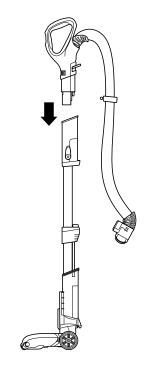
1 Place motorised floor nozzle on floor and insert wand, pressing it in until it clicks securely into place.
