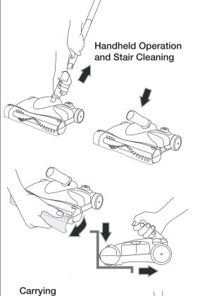
To avoid spilling dirt from the Dust Tray do not carry the product 'nose down'. **Bin Empty**
