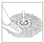
Step on the mop head fibres, with your foot at the edge of the green disc. Turn the handle so the screw joint is at a right angle to your foot.
