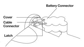
**WARNING:** NEVER touch both the metal battery contacts at the same time with any metal objects as this may create sparks that can cause small burns.
