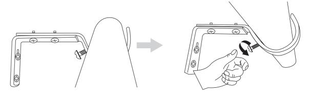
Tighten the bracket screw
