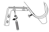
Loosen screws slightly, adjust to required extension, re-tighten screws.
