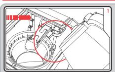
Fill the Water Reservoir (9) with cold water using the Internal Water Gauge (3) for guidance. Fill water to the required amount of cups that you would like to produce. Do not exceed the maximum 12 cups level.
