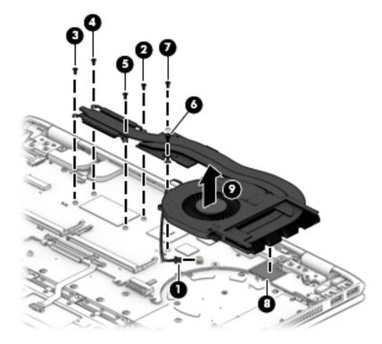
5. Thoroughly clean the thermal material from the surfaces of the fan/heat sink assembly and the system board components each time the fan/heat sink assembly is removed. Replacement thermal material is included with the fan/heat sink assembly and system board spare part kits.
