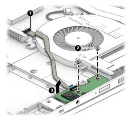
Reverse this procedure to install the audio/power button board.
