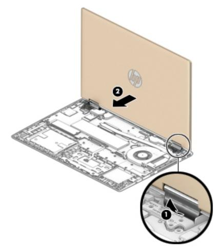
Reverse this procedure to install the display assembly.
