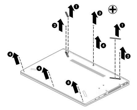
5. Using a plastic tool, starting near a hinge under the display, pry the bottom cover up to remove it (2).
