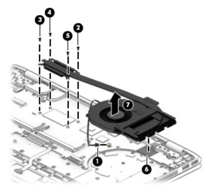
10. Thoroughly clean the thermal material from the surfaces of the fan/heat sink assembly and the system board components each time the fan/heat sink assembly is removed. Replacement thermal material is included with the fan/heat sink assembly and system board spare part kits.
