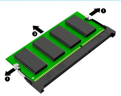
**NOTE:** Memory modules are designed with a notch to prevent incorrect insertion.
