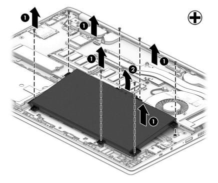
Reverse this procedure to install the battery.
