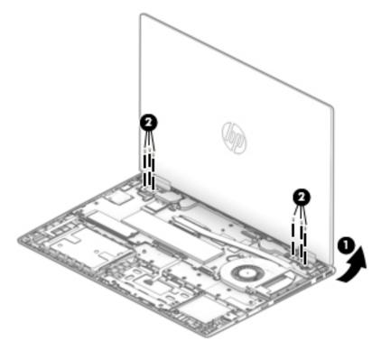
8. With display open about 270 degrees (1), pull the display away to separate it from of computer (2).
