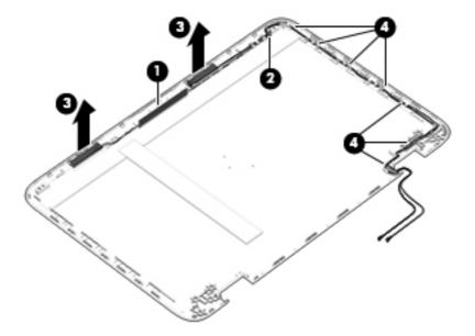
e. Remove the WLAN antenna cables and transceivers.
