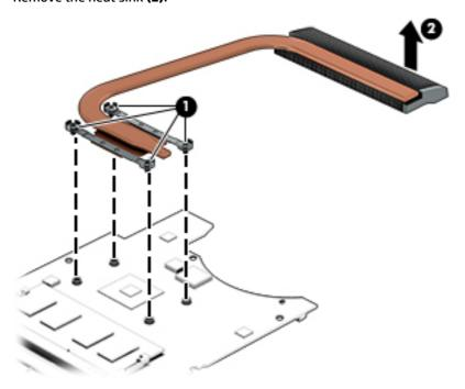
NOTE: The thermal material must be thoroughly cleaned from the surfaces of the heat sink and the system board each time the heat sink is removed. Thermal paste is used on the processor (1) and the heat sink section (2) that services it.
