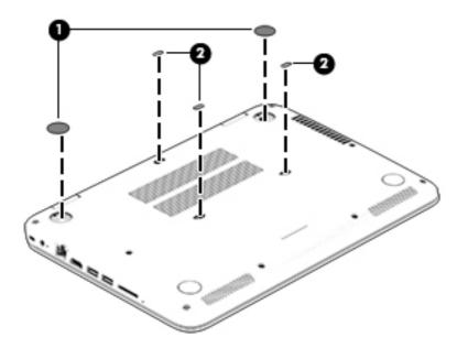
5. Remove the 13 Phillips PM2.4×5.7 screws that secure the keyboard/top cover to the bottom cover.
