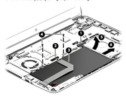
Reverse this procedure to install the battery.
