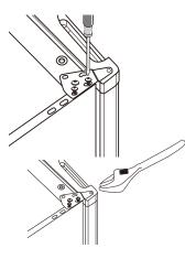
9. Put the top cover back and fix it in place with the screws.
