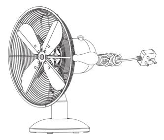
4, Mount Front Safety Grille onto Rear Grille by hanging the top hook clip of front guard over the top of the Rear Grille. Close the clasps all around the grille.
