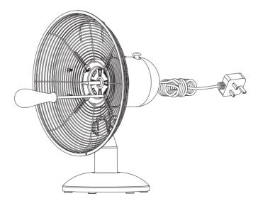
3, Discard plastic sleeve on shaft.Install the blade onto the shaft until the retaining pin fits into the notch on the blade, then use the Screw to fixed it and tighten (but do not over tighten)
