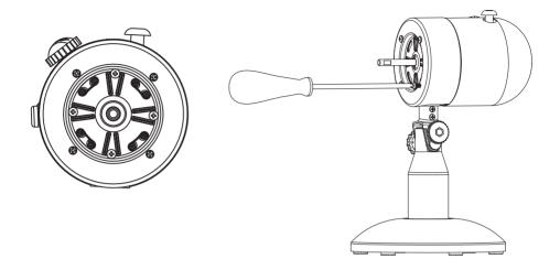
2, Set the rear grille in the proper position with the handle up.Let the four screw go through rear guard's hole and tighten (but do not over tighten).
