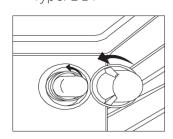
Replacement lamps are available from our Support Team. Replace the glass cover and reconnect the oven to the mains power supply.
