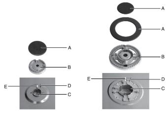
These parts can be removed for cleaning periodically. After cleaning, they must be well dried and correctly replaced. It is important to check that the burner bowl and cap have been correctly positioned. Failure to do so can cause serious problems.
