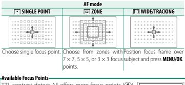
TTL contrast-detect AF offers more focus points ((1))than intelligent hybrid AF  $((\mathbf{2}))$ , which combines phase-detection with TTL contrast-detect AF.
