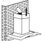
ii. Sliding the chimney to adjust the chimney height. When the height you required is reached, then hang the fixing hole to the fixing screws as showed in below pictures.
