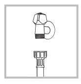
1. Connect the supply pipe by screwing it to a cold water tap using a 3/4 threaded connection (see figure). Before performing the connection, allow the water to run freely until it is perfectly clear.
