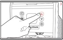
The default time will show 12am. Use the Up (14) and Down (15) buttons to change the time and press Program (11) to confirm.
