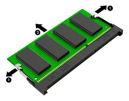
To protect a memory module after removal, place it in an electrostatic-safe container.
