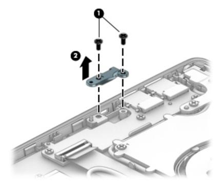
Reverse this procedure to install the lock bracket.
