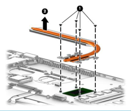
NOTE: The thermal material must be thoroughly cleaned from the surfaces of the heat sink and the system board components each time the heat sink is removed. Replacement thermal material is included with the heat sink and system board spare part kits.
