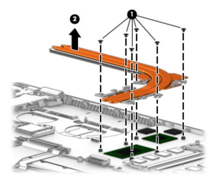
UMA graphics: In the order indicated on the heat sink, remove the four Phillips M2.0 × 2.5 screws (1) that secure the heat sink to the system board.
