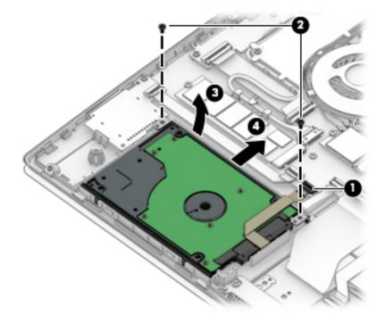
4. If it is necessary to disassemble the hard drive, pull the rubber bracket away from the hard drive (1), remove the two Phillips M3.0 × 3.0 screws (2), remove the metal bracket (3), and then disconnect the hard drive cable (4).
