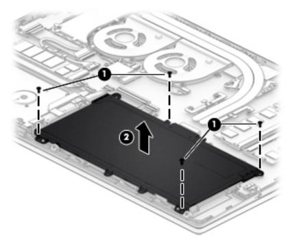
Reverse this procedure to install the battery.
