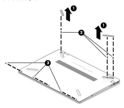
3. Starting under the hinges (1), use a thin plastic tool to disengage the bottom cover from the computer (2).
