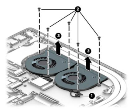
Reverse this procedure to install the fan(s).
