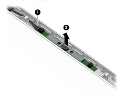
**c.** The camera/microphone module is available using spare part number L28107-001 for FHD infrared camera/microphone modules.
