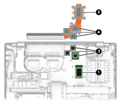
**UMA memory:** Thermal paste is used on the processor (1) and the heat sink (2).
