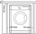
air inlets on the rear panel are not blocked or obstructed.
