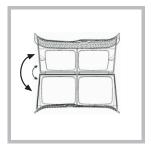
2. Clean the fluff off the filter and replace it correctly. Ensure that the filter is pushed fully home.
