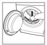
The filter is located behind of the dryer seal (see *Picture*).
