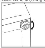
2. If the floor is not perfectly level, compensate for any unevenness by tighténing or loosening the adjustable front feet (see figure); the angle of inclination, measured in relation to the worktop, must not exceed 2°.
