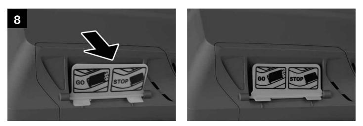
Your mower may be fitted with a grass full indicator. This is a small red flap on the top side of the grass collector.
