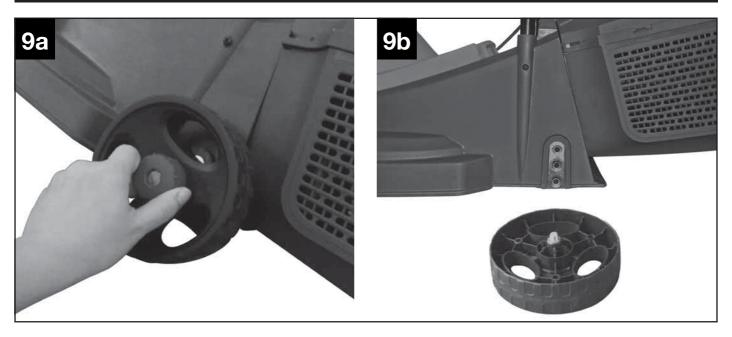
**IMPORTANT**! Set the cutting height only when the motor is switched off and the power cable has been disconnected.
